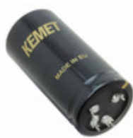
ALF20G562EF100 KEMET CAP ALU 5600UF 20% 100V PRESSFIT
