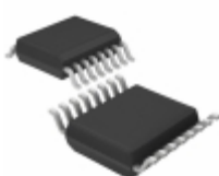
AD7785BRUZ-REEL ADI (Analog Devices, Inc.) IC ADC 20BIT 3CH LN LP 16- TSSOP
