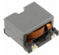
CDEP147NP-5R9MC-73 Sumida America Components Inc. FIXED IND 5.9UH 10A 9.85 MOHM
