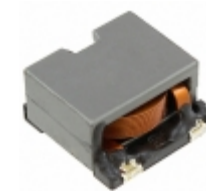
CDEP147NP-4R7MC-95 Sumida America Components Inc. FIXED IND 4.7UH 12.5A 6.03 MOHM
