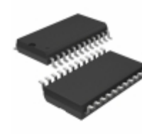
CY7B9910-2SC Cypress Semiconductor IC CLK BUFF SKEW 8OUT 24SOIC
