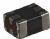
ACM4532-601-2P-T001 TDK Corporation CMC 1.5A 2LN 600 OHM SMD
