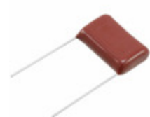
ECQ-E6474KFB Panasonic Electronic Components CAP FILM 0.47UF 10% 630VDC RAD
