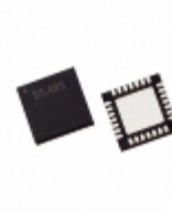
CP2109-A01-GMR Silicon Labs IC BRIDGE USB TO UART QFN
