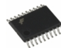
74LVTH273MTC AMI Semiconductor / ON Semiconductor IC FF D-TYPE SNGL 8BIT 20TSSOP
