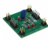
ADP7185-ADJ-EVALZ ADI (Analog Devices, Inc.) EVAL BOARD FOR ADP7185 -2.5V
