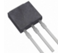
KSD1221GTU AMI Semiconductor / ON Semiconductor TRANS NPN 60V 3A I-PAK
