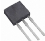
KSD12210TU AMI Semiconductor / ON Semiconductor TRANS NPN 60V 3A I-PAK
