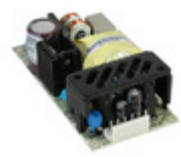
RPD-60B MEAN WELL AC/DC CONVERTER 5V 24V 54W
