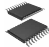
AT25320T2-10TC-2.7 Microchip Technology IC EEPROM 32KBIT 3MHZ 20TSSOP
