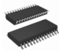
AT28C64X-25SI Microchip Technology IC EEPROM 64KBIT 250NS 28SOIC
