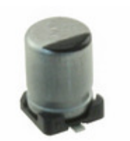
EEE-FT0J101AR Panasonic Electronic Components CAP ALUM 100UF 20% 6.3V SMD
