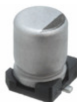
EEE-FT0J221AR Panasonic Electronic Components CAP ALUM 220UF 20% 6.3V SMD
