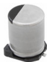
EEE-FT1A102AP Panasonic Electronic Components CAP ALUM 1000UF 20% 10V SMD
