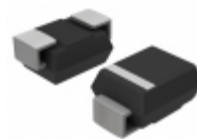
SMCJ408CA Bourns Inc. TVS DIODE 408VWM 658VC DO214AB
