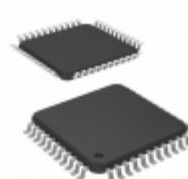
AT89S53-24AC Microchip Technology IC MCU 8BIT 12KB FLASH 44TQFP
