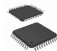
AT89S53-24AI Microchip Technology IC MCU 8BIT 12KB FLASH 44TQFP
