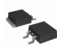
IRFS4615PBF Infineon Technologies MOSFET N-CH 150V 33A D2-PAK
