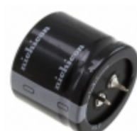
LLG2Z102MELB25 Nichicon CAP ALUM 1000UF 20% 180V SNAP
