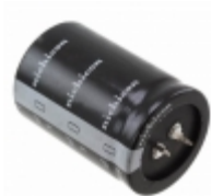
LLG2W821MELC50 Nichicon CAP ALUM 820UF 20% 450V SNAP
