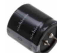
LLG2W471MELC35 Nichicon CAP ALUM 470UF 20% 450V SNAP
