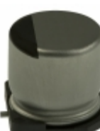
EEV-HA1A102P Panasonic Electronic Components CAP ALUM 1000UF 20% 10V SMD
