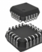
MC10H162FN ON Semiconductor IC DECODER BIN 1:8 20-PLCC
