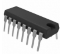
MC10H161P ON Semiconductor IC DECODER BIN 1:8 16-DIP
