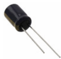
EEU-FC0J471BJ Panasonic Electronic Components CAP ALUM 470UF 20% 6.3V RADIAL
