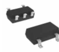
MIC5253-2.6BC5 Microchip Technology IC REG LDO 2.6V 0.1A SC70-5
