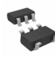
FHP3132IS5X AMI Semiconductor / ON Semiconductor IC OPAMP VFB 260MHZ RRO SOT23-5
