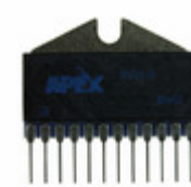
PA13EE Apex Microtechnology IC OPAMP 90V 10A PSIP
