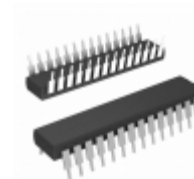
PIC16C55A-20I/SP Microchip Technology IC MCU 8BIT 768B OTP 28SDIP
