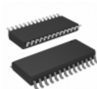
PIC16C55A-20/SO Microchip Technology IC MCU 8BIT 768B OTP 28SOIC
