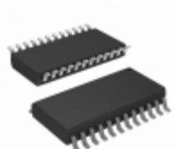
STP16CP596MTR STMicroelectronics IC LED DRIVER LINEAR 50MA 24SO
