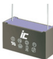
MPXB155K305H Illinois Capacitor CAP FILM 1.5UF 10% 305VAC RAD
