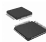
PIC16F19195T-I/PT Micrel / Microchip Technology IC MCU 8BIT 14KB FLASH 64TQFP
