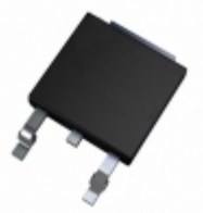
IXCY20M35A IXYS IC CURRENT REGULATOR DPAK
