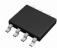
BR93G76FVJ-3AGTE2 Rohm Semiconductor IC EEPROM 8KBIT 3MHZ 8TSSOP
