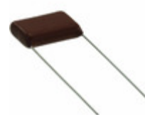
ECQ-E6124JFW Panasonic Electronic Components CAP FILM 0.12UF 5% 630VDC RADIAL
