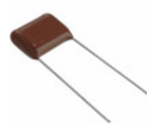
ECQ-E4394JFW Panasonic Electronic Components CAP FILM 0.39UF 5% 400VDC RADIAL
