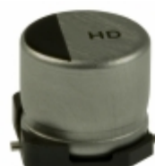
EEV-HD1H100P Panasonic Electronic Components CAP ALUM 10UF 20% 50V SMD
