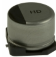
EEV-HD1E470P Panasonic Electronic Components CAP ALUM 47UF 20% 25V SMD
