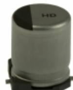
EEV-HD1C101P Panasonic Electronic Components CAP ALUM 100UF 20% 16V SMD
