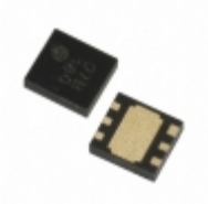
XC6121A736ER-G Torex Semiconductor Ltd IC WATCHDOG TIMER 6-USP
