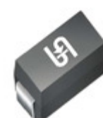
1SMA5939HR3G TSC (Taiwan Semiconductor) DIODE ZENER 39V 1.5W DO214AC
