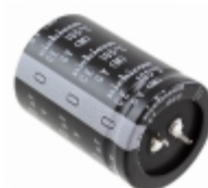
LGY2W331MELC Nichicon CAP ALUM 330UF 20% 450V SNAP
