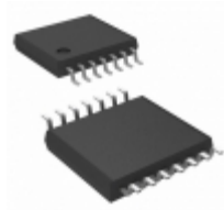
AD8302ARUZ-RL7 Analog Devices Inc. IC DETECT GAIN PHASE 14-TSSOP TR
