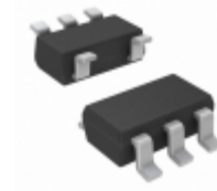
MCP1804T-A002I/OT Microchip Technology IC REG LDO 10V 0.15A SOT23-5
