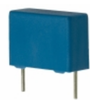
B32652A4474K289 EPCOS (TDK) CAP FILM 0.47UF 10% 400VDC RAD
