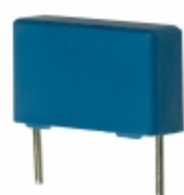
B32652A4683K000 EPCOS CAP FILM 0.068UF 10% 400VDC RAD
