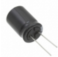
URS2D101MHD1TN Nichicon CAP ALUM 100UF 20% 200V RADIAL
