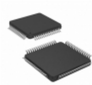
PIC32MX664F064HT-V/PT Microchip Technology IC MCU 32BIT 64KB FLASH 64TQFP
