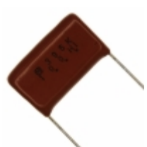
ECQ-E6334KF Panasonic Electronic Components CAP FILM 0.33UF 10% 630VDC RAD
