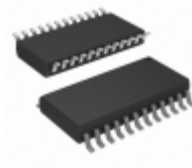
ICL3207ECB-T Intersil IC 5DRVR/3RCVR RS232 3V 24-SOIC
