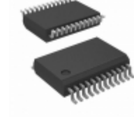
ICL3207ECAZ-T Intersil IC 5DRVR/3RCVR RS232 3V 24-SSOP
