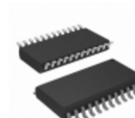
ICL3207CBZ Intersil IC 5DRVR/3RCVR RS232 3V 24-SOIC
