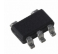
MIC5256-2.8YM5-TR Microchip Technology IC REG LDO 2.8V 0.15A SOT23-5
