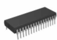
AT27C080-90DC Microchip Technology IC EPROM UV 8MBIT 90NS 32CDIP
