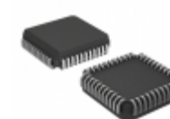
AT27C1024-12JI Microchip Technology IC OTP 1MBIT 120NS 44PLCC
