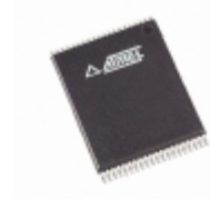
AT27C1024-12VC Microchip Technology IC OTP 1MBIT 120NS 40VSOP
