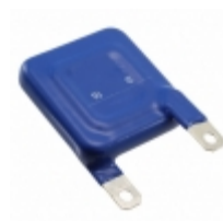
LS40K460QPK2 EPCOS (TDK) VARISTOR 750V 40KA CHASSIS
