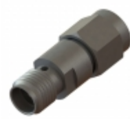
SF0929-6200-155 Amphenol SV Microwave ATTENUATOR 18GHZ 15.5DB 50OHM
