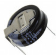
DXJ-5R5H224U Elna America CAP 220MF -20% +80% 5.5V T/H
