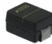
CU3225K250G2K1 EPCOS (TDK) VARISTOR 390V 400A 3225
